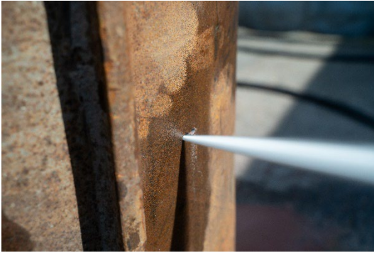
caption: Abrasive cutting means cutting without sparkles. The cutting power is created by high-pressure water and small abrasive particles that goes among the water flow. As a result, the jet penetrates materials. Alt text: Abrasive cutting through a material
